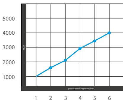
The Normal liter/hour air consumption depends on applied pressure, users number and point connection tube diameter (be careful in case of spray, nozzle diameter must be kept into account).
