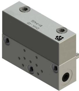
The by-pass element is dimensionally identical to the metering model, but does not contain the piston. It has the function of creating a reserve position when the number of outlets change.
