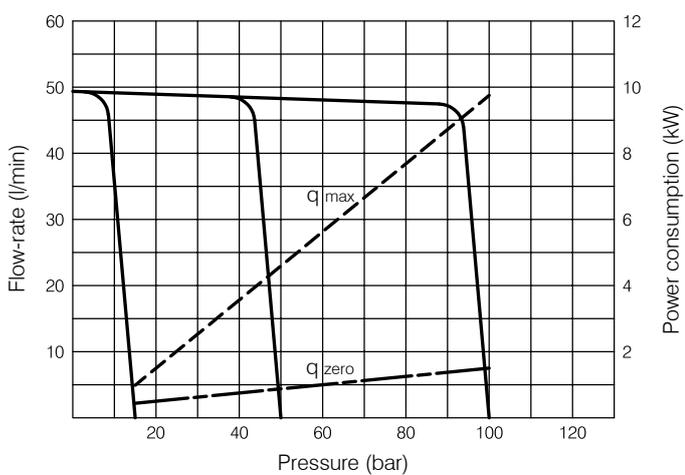
Indicative values measured on Berarma test stand, referring to 1500 rpm with HM hydraulic oil according to ISO 6743-4, ISO VG 46 according to ISO 3448, temperature 40 °C. Sound level meter placed 1 meter from the pump with flexible coupling.
