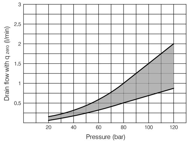
Indicative values measured on Berarma test stand, referring to 1500 rpm with HM hydraulic oil according to ISO 6743-4, ISO VG 46 according to ISO 3448, temperature 40 °C. Sound level meter placed 1 meter from the pump with flexible coupling.
