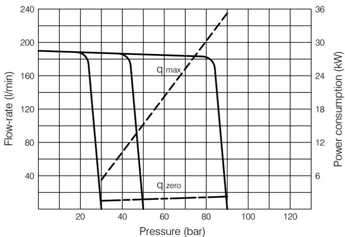
Indicative values measured on Berarma test stand, referring to 1500 rpm with HM hydraulic oil according to ISO 6743-4, ISO VG 46 according to ISO 3448, temperature 40 °C. Sound level meter placed 1 meter from the pump with flexible coupling.
