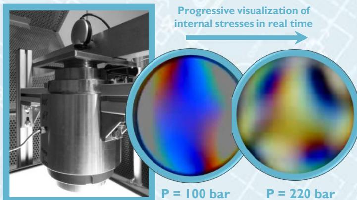
**Control of internal stresses inside of a quartz window**
