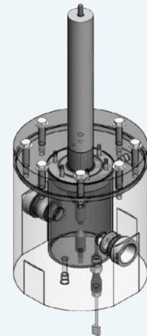
**I axis optical cell 400 bar / 1000 V**
