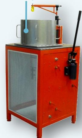
**Corrosion testing autoclave**
